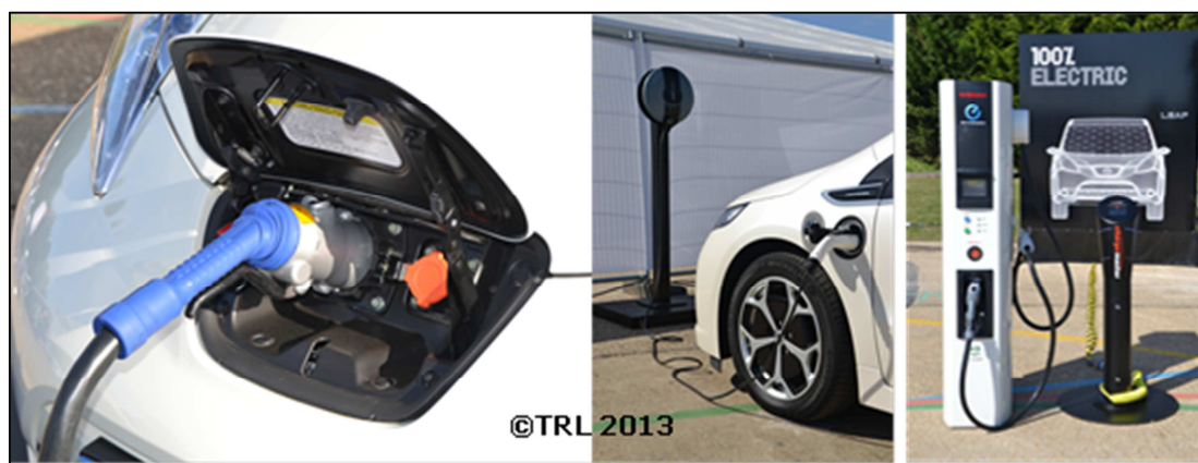
Figure1: Examples of plug-in charging vehicles and chargers
