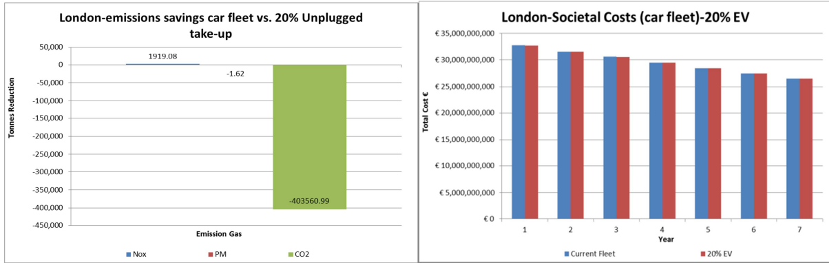
Figure 41 - Reduced emissions (a) and resulting societal cost reductions (b) - London cars 20% EV This change in fleet composition would reduce Carbon Dioxide emissions by just over 400,000 tonnes.
