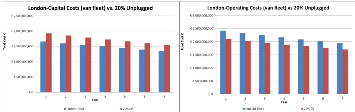
Figure 54 - Fleet impact on capital (a) and operating costs (b): 20% Unplugged take-up rate
