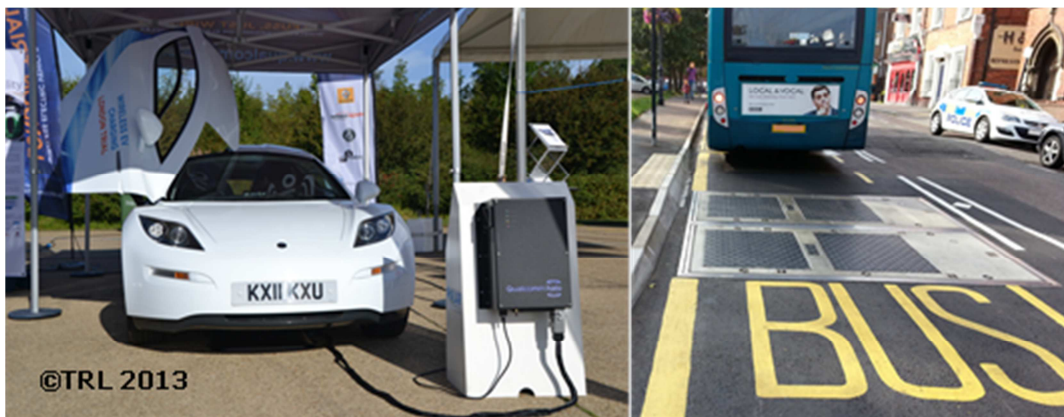
Figure 3: Examples of WPT Charging, for a car using a mat (left), WPT charging for a bus built into the road surface (right)
