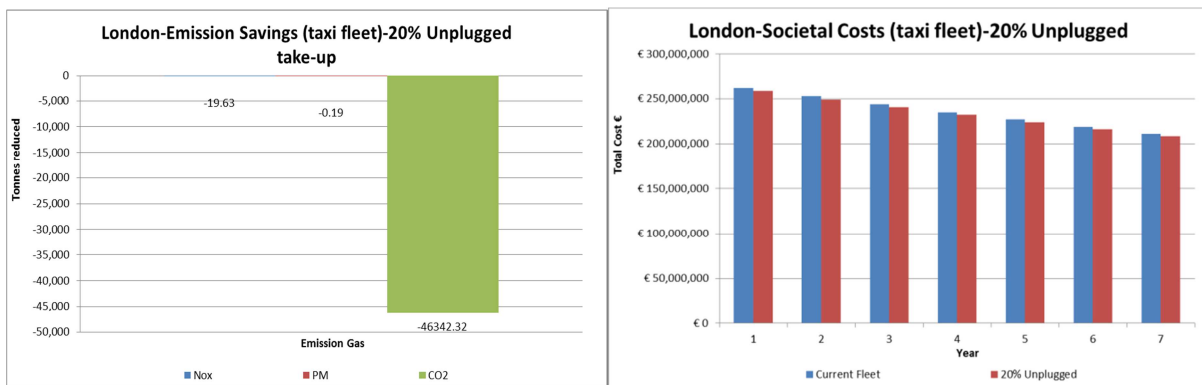
Figure 66 - Reduced emissions in tonnes (a) and resulting societal cost reductions (b) - London taxis 20% Unplugged
